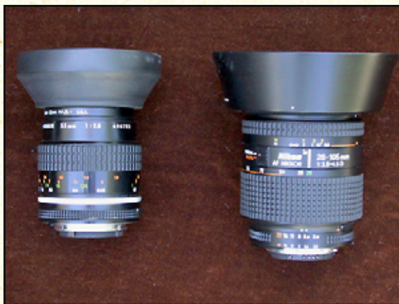
fig.7 Select a lens that will minimize distortion. this can be a macro lens or a zoom lens used at 85 mm or longer.
