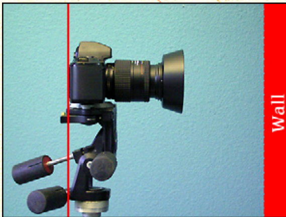
fig.5 With your camera mounted to the tripod, set the tripod's head adjustments so that the back of the camera is parallel to the wall. This will eliminate the keystone affect. see fig. 12
